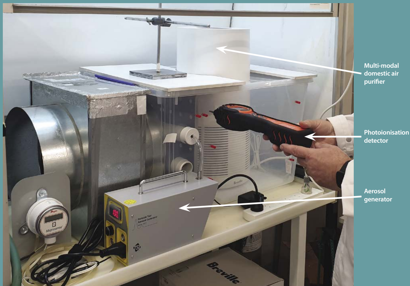
Figure 1: The domestic air purifier located in the test chamber. A 10.6 eV photoionisation detector for vapours is also illustrated on the right.
